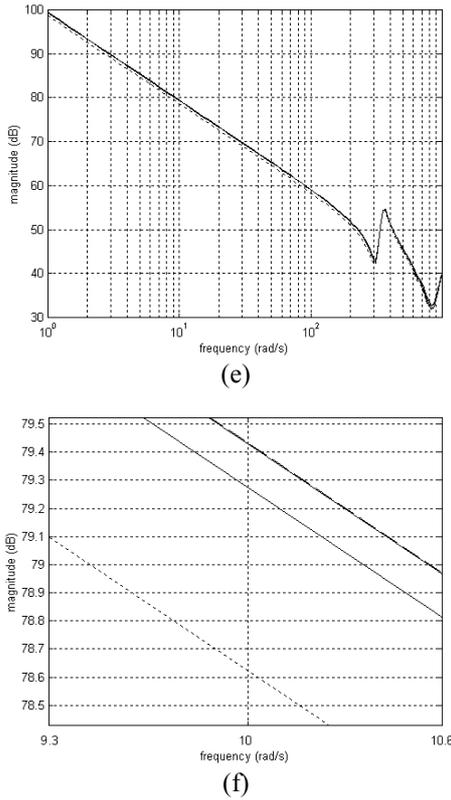
Fig.7 Plot of realistic performance boundaries (solid-line),  $Z_h(z)$  (long-dash-line) and  $Z_{h\_vc}(z)$  (short-dash-line) when the virtual environment parameters are (a)  $b_e = 0.1$  N.s/m,  $k_e = 10$  N/m, (b) enlarged figure of Fig.7a, (c)  $b_e = 1$  N.s/m,  $k_e = 1000$  N/m, (d) enlarged figure of Fig.7c, (e)  $b_e = 25$  N.s/m,  $k_e = 25000$  N/m, (f) enlarged figure of Fig.7e.
