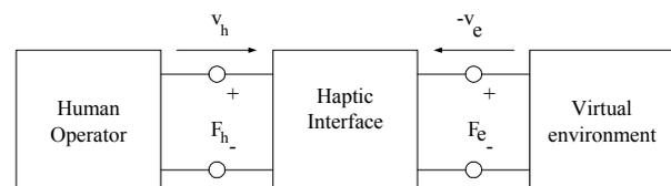
Fig.1 Two-port network of a haptic interface.
