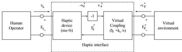
Fig.2 Two-port network of an impedance display haptic interface with a virtual coupling.
