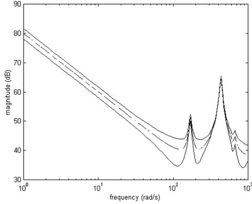
Fig.5 Realistic performance boundaries of a haptic interaction
