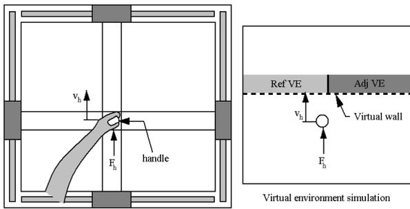
Fig.6 Virtual wall simulation. (Note that Ref VE and Adj VE are reference and adjustable virtual environment respectively)
