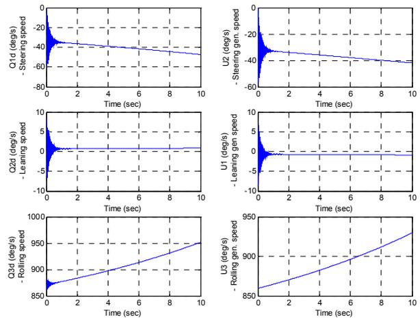
Fig.4 Time Derivative of Generalized Coordinates  $\dot{q}_i$  and Generalized Speeds  $u_i$  of a One-Wheel Robot
