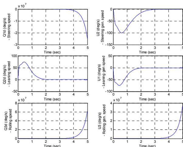
Fig.7 Time Derivative of Generalized Coordinates  $\dot{q}_i$  and Generalized Speeds  $u_i$  of a Rolling Disk
