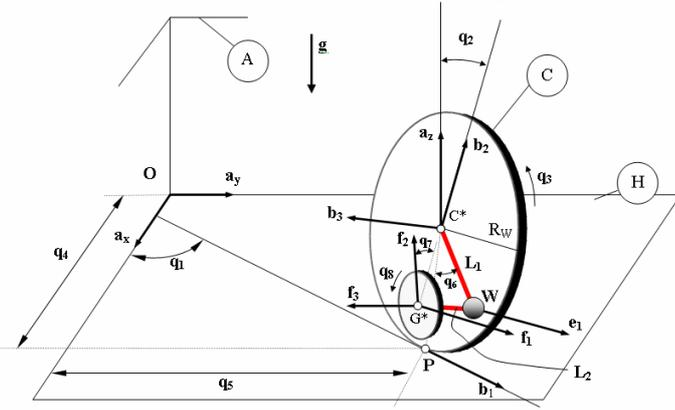
Fig.1 Coordinate Assignment for a One-Wheel Robot Rolling on Horizontal Plane
