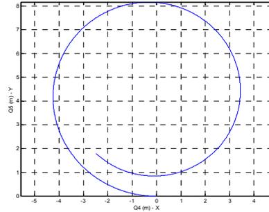
Fig.3 Position of a Contact Point ( $q_4, q_5$ ) of a One-Wheel Robot on X-Y Plane
