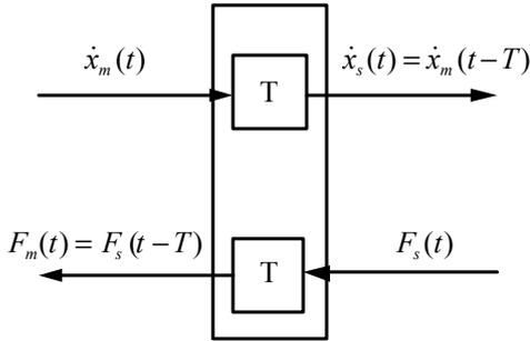
**Figure 1:** A model of single delayed standard communication
