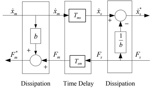
**Figure 2:** The standard communication with sufficient dissipation
