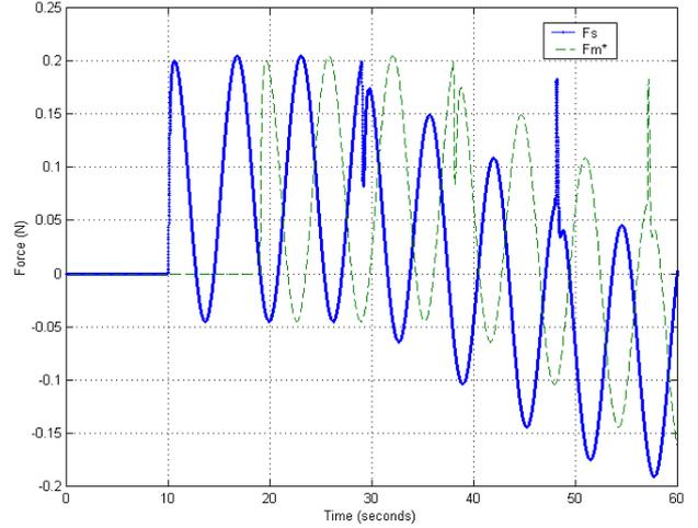
**Figure 7:** The result of adaptive  $b_m(t)$  implementation with constant delay of 10 s.
