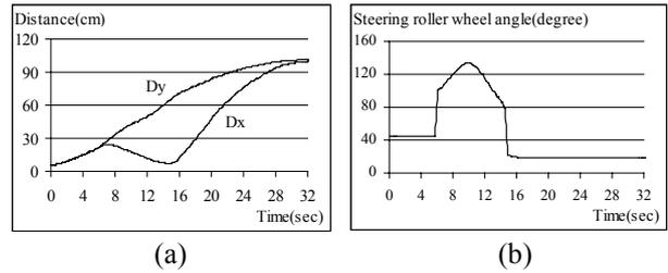
Figure 17 (a) Positions of an object2 vs. time (b) Steering roller wheel angle of an object2 vs. time
