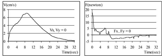
Figure 12 (a) Velocity profiles of an objects3 (b) Driving force of an object3
