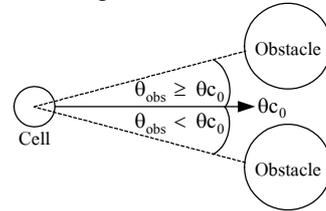
Figure 3 Criteria for setting the steering roller wheel angle
