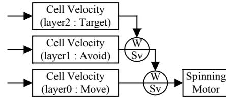
Figure 5 Diagram for subsumption-based control for the spinning roller wheel
