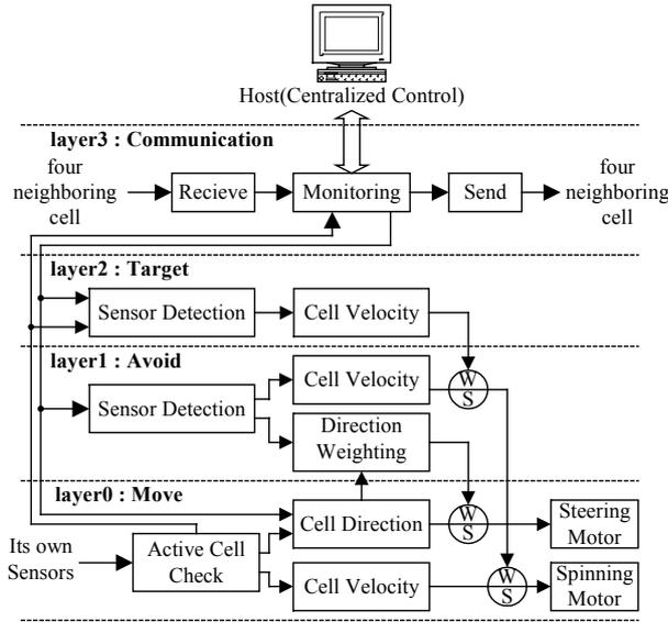
Figure 2 Four-layer control of subsumption architecture
