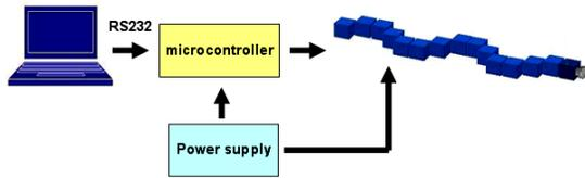
Fig. 3 A system diagram of the snake robot
