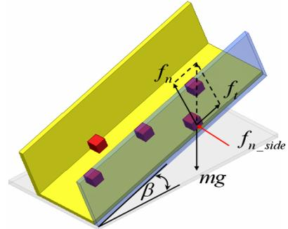
Fig. 5 The force diagram at the non-slipped contact point
