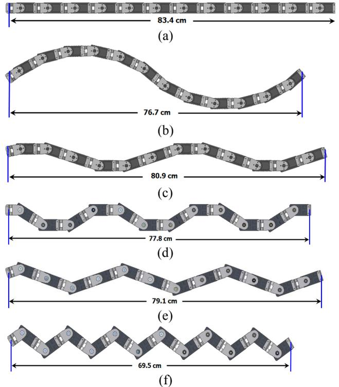
Fig. 10 The geometrical effective length of the robot along the pipe axis (a) full length (b) case I (c) case II (d) case III.I (e) case III.II (f) case IV
