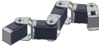
Fig. 2 CAD model of a modular snake robot
