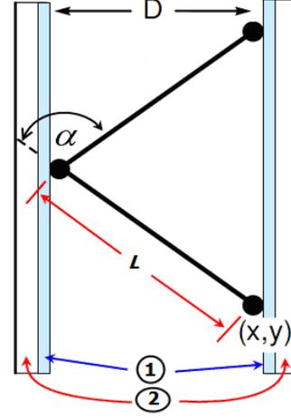
Fig. 8 The geometrical relationship of the basis angle and pipe with (1) indicates the compliant inner wall of the pipe, (2) indicates the rigid outer wall of the pipe.
