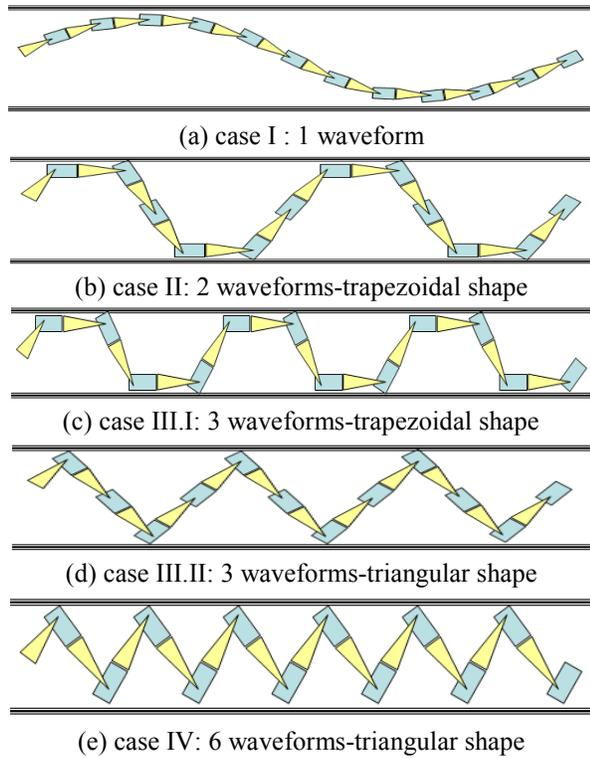
Fig. 9 Five cases of motion shape in the experiment a) case I b) case II c) case III.I d) case III.II e) case IV
