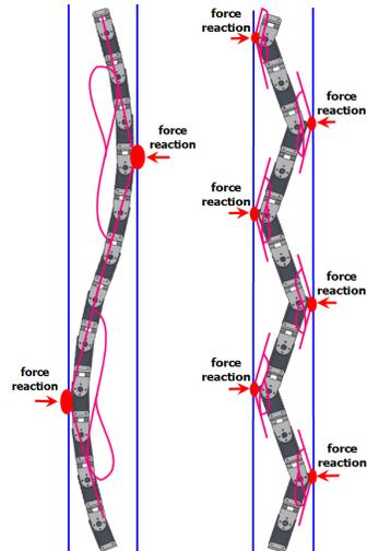
Fig. 6 The relationship between forces generated by motion shape and friction cone of the surface that resulted in the non-slipped contact points
