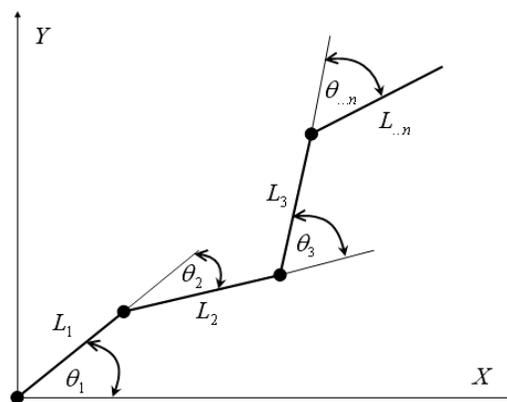
Fig. 1 A snake robot kinematics
