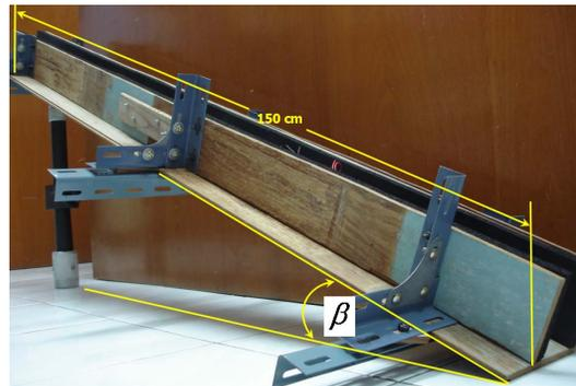
Fig. 11 The inclined pipe used in the experiment
