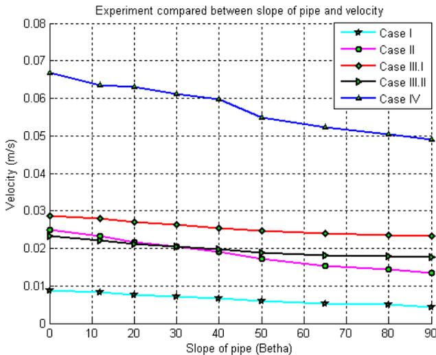
Fig. 13 The graph between crawling velocity (m/s) and inclined angle of the pipe (degrees) for each motion shape: case I, II, III.I, III.II and IV
