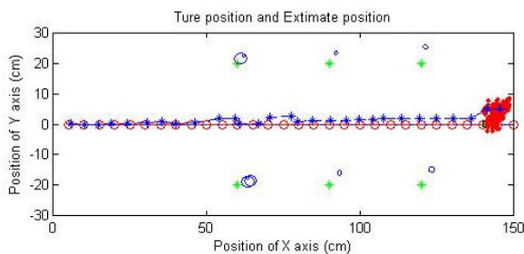
Figure 10. Estimated position of the UGV without information from the UAV: (o) is the way-points, (\*) is the estimated position from FastSLAM.
