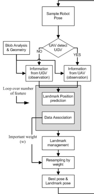
Figure 6. Flow chart of the proposed FastSLAM algorithm
