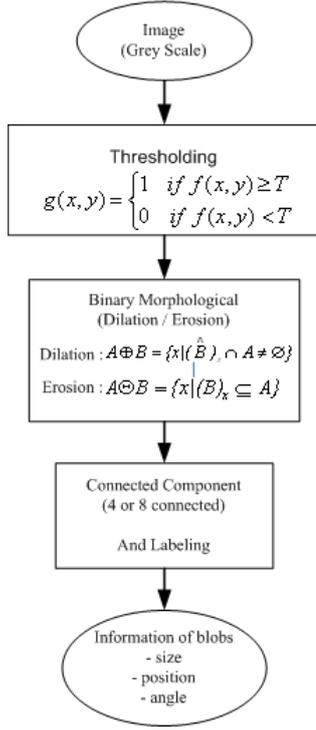
Figure 2. Diagram of blob analysis algorithm
