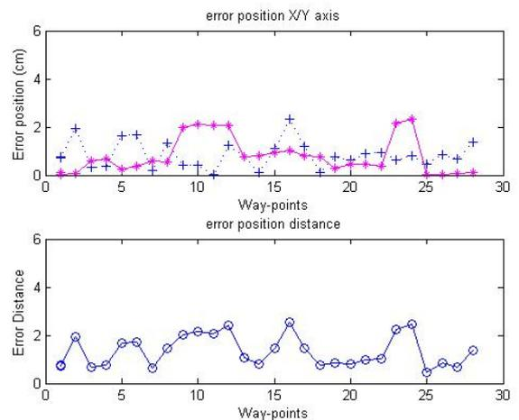
Figure 13. Position error between the way-points and the estimate position in X/Y axis: (+) is error X axis and (\*) is error Y axis, and distance error between the way-points and the estimated position
