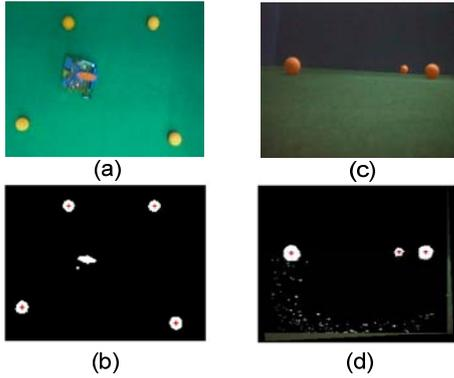
Figure 3. Raw Image: Top view (a) and Front view (c). Processed image by blob analysis: Top view (b) and Front view (d).
