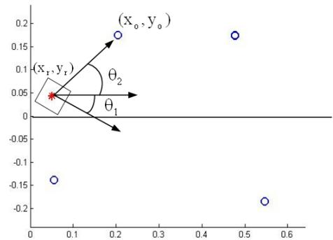
Figure 4. Estimation of distance and angle between the ground robot and the landmark from the top view.
