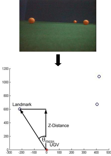
Figure 5. Estimation of distance and angle between the ground robot and the landmark from the front view image
