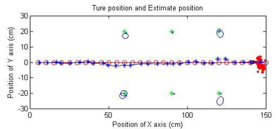
Figure 12. Estimated position of the UGV with the combined information from the UAV: (o) is the way-points, (\*) is the estimated position from FastSLAM.
