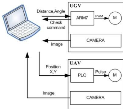
Figure 9. System block diagram
