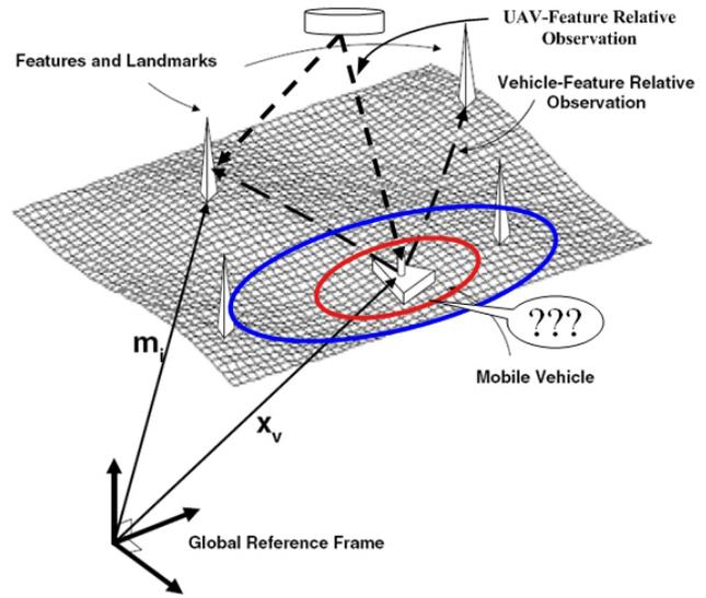
Figure 1. The conceptual diagram of air-ground cooperative localization
