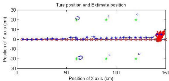
Figure 10. Estimated position of the UGV without information from the UAV: (o) is the way-points, (\*) is the estimated position from FastSLAM.
