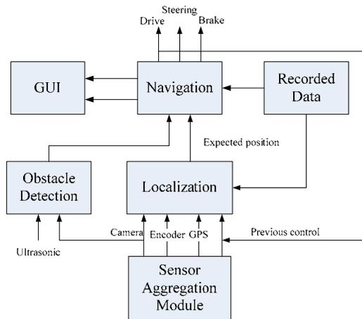
**Fig. 5** System diagram for the autonomous navigation system
