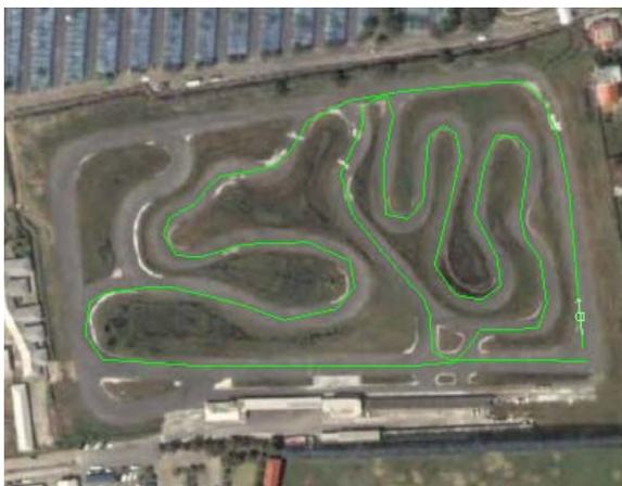
**Fig. 6** GUI shows the current estimated position of the vehicle (green rectangle on the lower right corner) on the recorded trajectory (green line)
