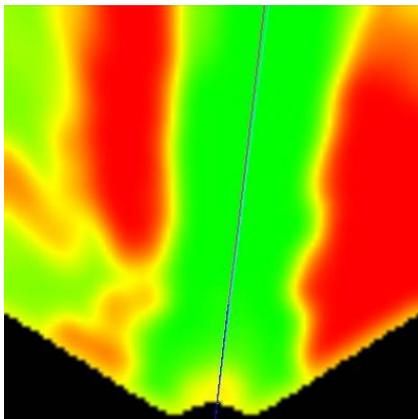
**Fig. 9** the projected images of the avoidance value (green represents a low avoidance value and red represents a high avoidance value)
