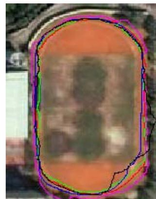
**Fig. 11** the GPS position of four GPS's and the estimated position overlaid on top of the satellite image of the KMUTT football field during the teaching phase
