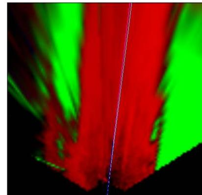
**Fig. 8** the projected images from the left and right cameras after the scoring process (the red-channel represents the score associated with the dirt road, the green-channel represents the score associated with the grass, the blue line indicates the optimal chosen path)
