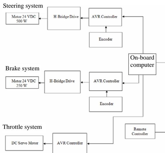
**Fig. 2** Actuation System
