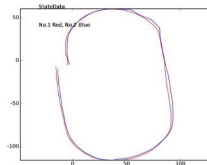
**Fig. 10** the estimated position in the teaching (red line) and autonomous playback (blue line) phase
