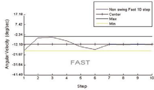
Fig. 5 Graph of the angular velocity during the fast-walking gait with no swing arm (experiment 3).
