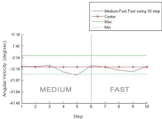
Fig. 10 Graph of the angular velocity during the transition from medium to fast walking gait with no swing arm in medium and swing arm in fast (experiment 10).
