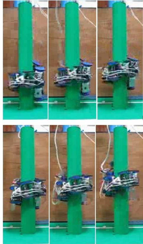
Fig. 13. Climbing experiment of the robot.
