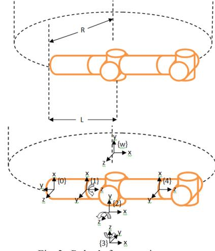
Fig. 2. Robot's frame assignment.
