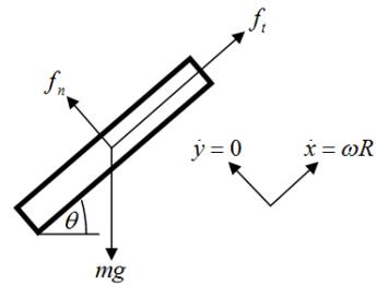
Fig. 5. Robot's wheel free body diagram.
