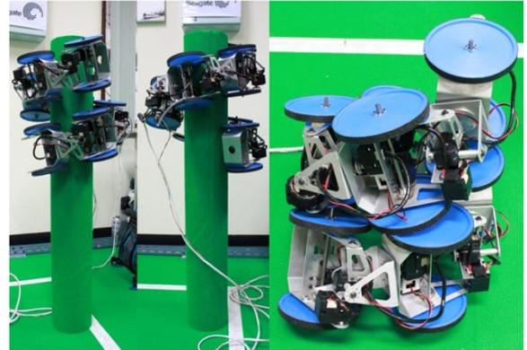
Fig. 8. (left, middle) The robot grasp testbed at 15 and 20 degree helical pitch, (right) Robot after controlled to form to helical shape.
