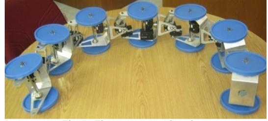
Fig. 7. The prototype snake robot.
