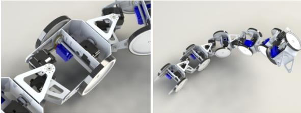
Fig. 6. CAD model of the modular snake robot.
