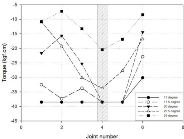
Fig. 10. The graph between holding torque of yaw angle and helical pitch angle.
