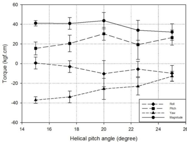
Fig. 9. The graph between mean and SD of holding torque in each axis of rotation and helical pitch angle.
