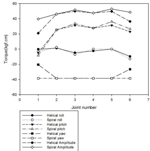
Figure 15. The comparison graph between helical path's holding torque and spiral path's holding torque with 15 degrees pitch angle.
