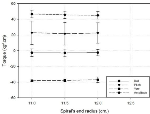
Figure 12. The graph between mean and SD of holding torque in each axis of rotation and spiral's end radius with 15 degrees pitch angle.
