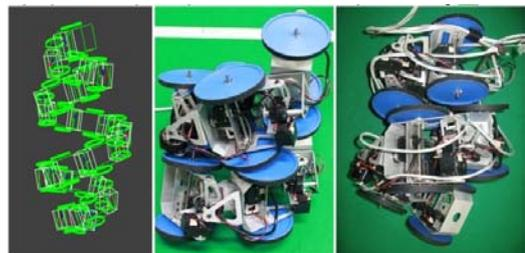
Figure 10. Simulation of spiral pose (left) and the real shape of helical pose (center) and spiral pose (right).
