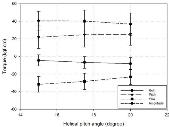
Figure 7. The graph between mean and SD of holding torque in each axis of rotation and helical pitch angle.
