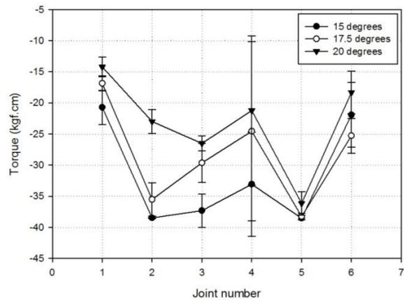
Figure 9. The graph of yaw's torque distribution along the robot's body and the helical pitch angle.
