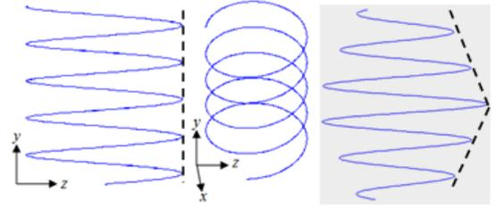
Figure 2. Circular helix path and spiral path.
