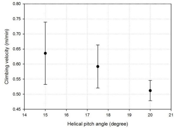
Figure 8. The graph between mean and SD of climbing velocity and helical pitch angle.
