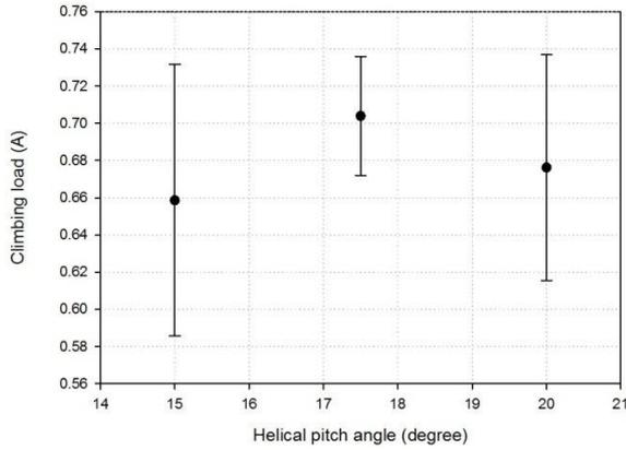
Figure 6. The graph between mean and SD of climbing load and helical pitch angle.
