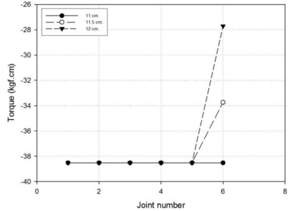
Figure 14. The graph between holding torque of yaw angle and spiral's end radius with 15 degrees pitch angle.
