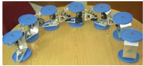
Figure 5. The prototype wheel-based modular snake robot.
