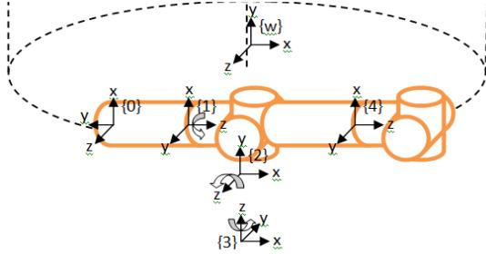
Figure 1. Robot's frame assignment.
