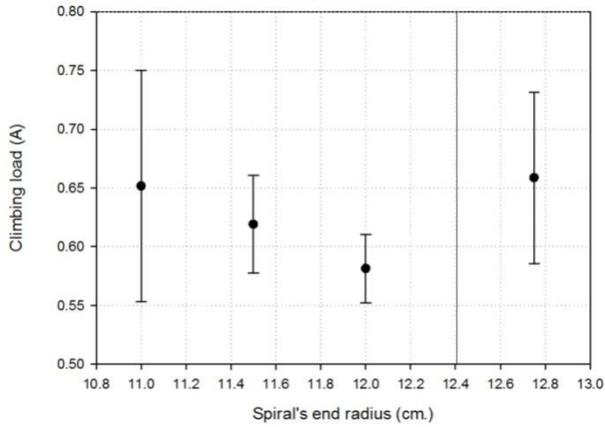
Figure 11. The graph between mean and SD of climbing load of spiral's end radius and helical climbing with 15 degrees pitch angle.
