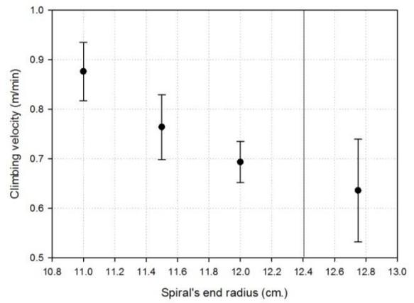
Figure 13. The graph between mean and SD of climbing velocity of spiral's end radius and helical climbing with 15 degrees pitch angle.
