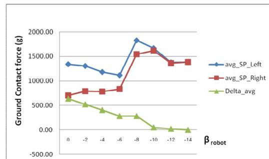
Fig. 7 Relationship between the difference of left/right ground contact force during the single support walking phase and the leaning angle
