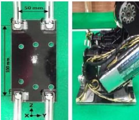
Fig.5 Force sensor attachment at the foot of the robot.
