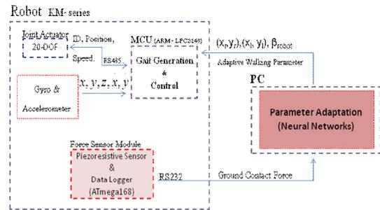
Fig. 11 The neural networks walking controller system diagram
