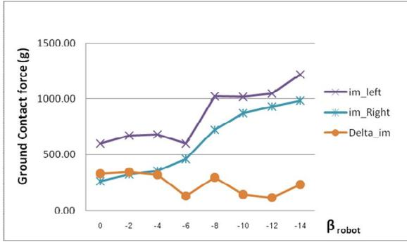
Fig. 8 Relationship between the difference of left/right ground contact force during the double support walking phase and the leaning angle
