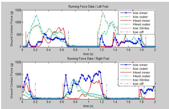
Fig. 13 The ground contacting force of one walking cycle after the body leaning angle was compensated by the proposed controller.
