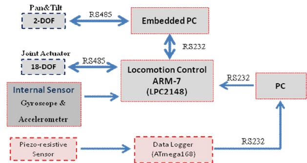
Fig. 2 KM's system diagram.
