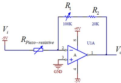
Fig.4 Inverting amplifier circuit.
