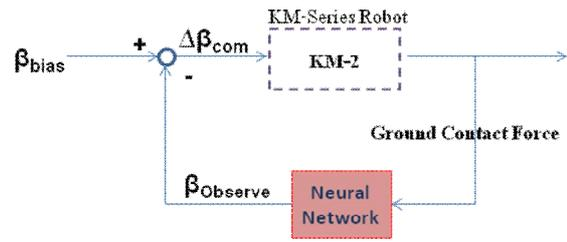
Fig.10 Neural Networks leaning angle compensator block diagram
