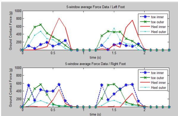
Fig. 9 Preprocessed force input to the neural networks of two walking cycles.
