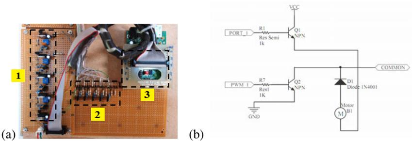
**Fig. 4.** (a) Tactile controller: 1) Row motor driver circuit 2) Column motor driver circuit 3) Arduino microcontroller (b) Schematic diagram of a tactile feedback driver
