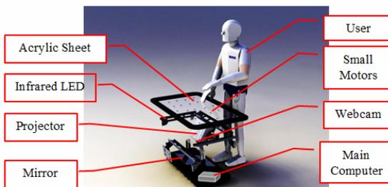
Fig. 2. System Components
