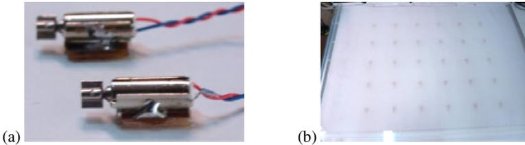
**Fig. 3.** (a) The implemented small DC motors. (b) Thirty motors mounted below the display.
